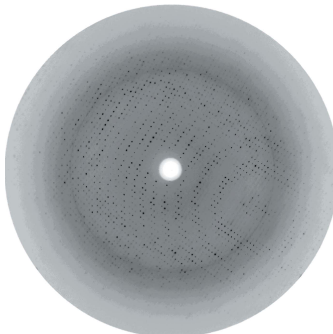
Figure 2 X-ray diffraction pattern from a scPvuII crystal. The detector edge corresponds to 2.3 \text{\AA} resolution.
